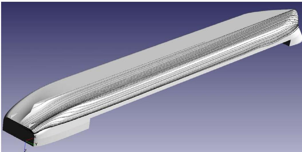
Fig. 3. Streamlines on Ship Hull. Speed 11.5 knots
