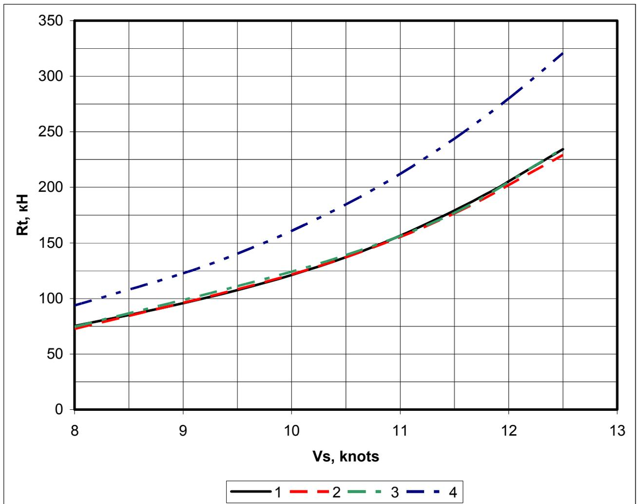
Fig. 8. Comparison Of The RSD19 Total Resistance With The Data of: 1 – model test; 2,3 – calculation with the CFD method; 4 – calculation by means of the Holtrop – Mennen method.
