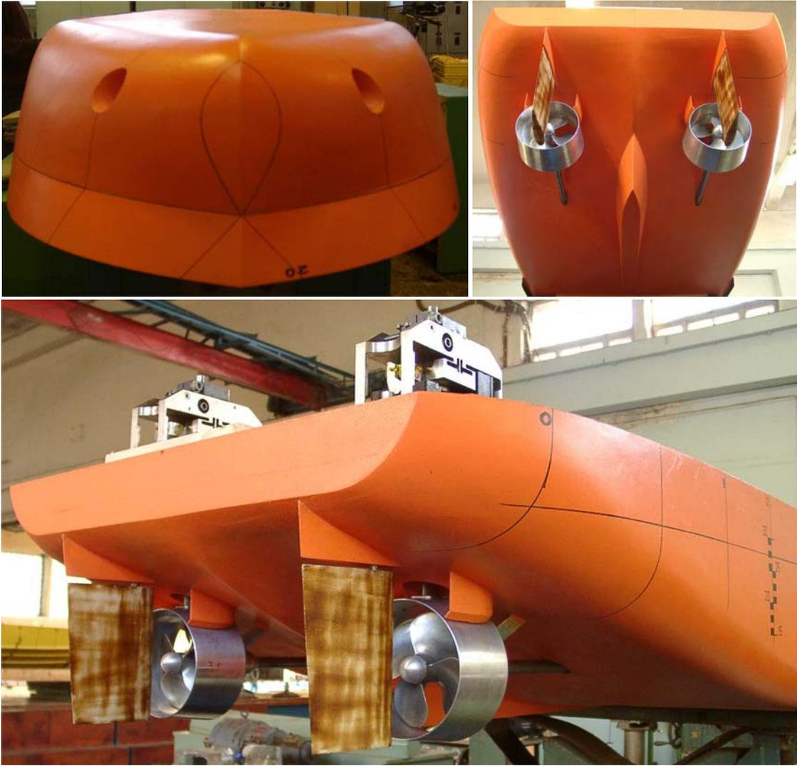
Fig. 7. Self-propelled Model Of The Ship (project RSD19) Made by Krylov Shipbuilding Research Institute.
