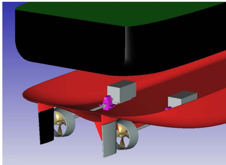
Fig 6. Three-dimensional Model of Propulsion System Arrangement
